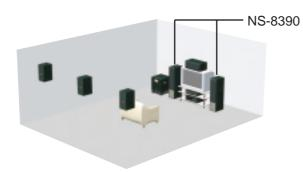
6.1-channel system consists of main L/R, center, rear L/R, rear center and LFE (low frequency effect, i.e. subwoofer) channels.
